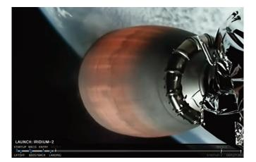
The Falcon 9's second-stage rocket fires one engine to position the Iridium NEXT payload in the correct orbital plane. Operational satellites orbit at an altitude of approximately 483 miles above the earth.
