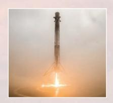
SpaceX's launch program was developed for rocket reusability. The images directly above and below show the landing of the first-stage rocket following the successful launch of Iridium NEXT satellites on June 25. This same first-stage was used on December 22 to launch another batch of Iridium NEXT satellites to space.
